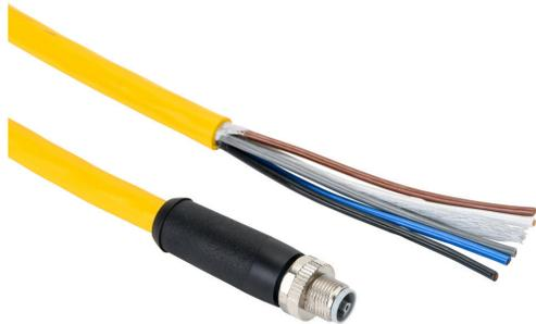
Murrelektronik power cable, M12 axial male L-coded to pigtail, 5-pole, 63 VDC, 16A, 14 AWG, TPE jacket, yellow, 6.5ft/2m cable length, IP65 IP67.
