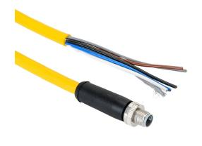
Murrelektronik power cable, M12 axial male L-coded to pigtail, 5-pole, 63 VDC, 12A, 16 AWG, TPE jacket, yellow, 49.2ft/15m cable length, IP65 IP67.
