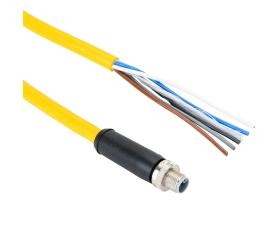
Murrelektronik power cable, M12 axial male L-coded to pigtail, 5-pole, 63 VDC, 12A, 16 AWG, TPE jacket, yellow, 24.6ft/7.5m cable length, IP65 IP67.
