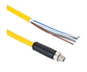
Murrelektronik power cable, M12 axial male L-coded to pigtail, 5-pole, 63 VDC, 12A, 16 AWG, TPE jacket, yellow, 16.4ft/5m cable length, IP65 IP67.
