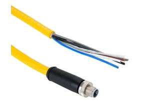
Murrelektronik power cable, M12 axial male L-coded to pigtail, 5-pole, 63 VDC, 12A, 16 AWG, TPE jacket, yellow, 9.8ft/3m cable length, IP65 IP67.
