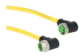
Murrelektronik connection cable, 7/8in - 16 UN2 90-degree male with male threads to 7/8in - 16 UN2 90-degree female with female threads, 4-pole, 600 VAC/VDC, 9A, 16 AWG, TPE jacket, yellow, unshielded, 9.8ft/3m cable length, IP68, power.
