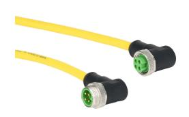
Murrelektronik connection cable, 7/8in - 16 UN2 90-degree male with male threads to 7/8in - 16 UN2 90-degree female with female threads, 4-pole, 600 VAC/VDC, 9A, 16 AWG, TPE jacket, yellow, unshielded, 3.2ft/1m cable length, IP68, power.
