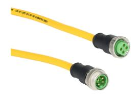
Murrelektronik connection cable, 7/8in - 16 UN2 axial male with male threads to 7/8in - 16 UN2 axial female with female threads, 4-pole, 600 VAC/VDC, 9A, 16 AWG, TPE jacket, yellow, unshielded, 32.8ft/10m cable length, IP68, power.
