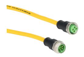
Murrelektronik connection cable, 7/8in - 16 UN2 axial male with male threads to 7/8in - 16 UN2 axial female with female threads, 4-pole, 600 VAC/VDC, 9A, 16 AWG, TPE jacket, yellow, unshielded, 16.4ft/5m cable length, IP68, power.
