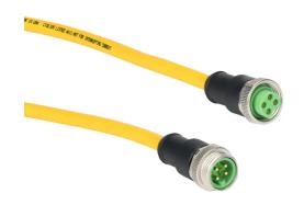
Murrelektronik connection cable, 7/8in - 16 UN2 axial male with male threads to 7/8in - 16 UN2 axial female with female threads, 4-pole, 600 VAC/VDC, 9A, 16 AWG, TPE jacket, yellow, unshielded, 3.2ft/1m cable length, IP68, power.
