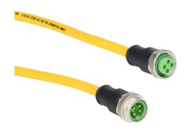
Murrelektronik connection cable, 7/8in - 16 UN2 axial male with male threads to 7/8in - 16 UN2 axial female with female threads, 4-pole, 600 VAC/VDC, 9A, 16 AWG, TPE jacket, yellow, unshielded, 0.9ft/0.3m cable length, IP68, power.
