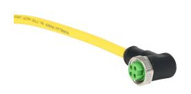
Murrelektronik connection cable, 7/8in - 16 UN2 90-degree female with female threads to Pigtail with European Color Code, 4-pole, 600 VAC/VDC, 9A, 16 AWG, TPE jacket, yellow, unshielded, 32.8ft/10m cable length, IP68, power.
