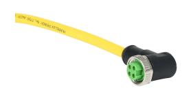
Murrelektronik connection cable, 7/8in - 16 UN2 90-degree female with female threads to Pigtail with European Color Code, 4-pole, 600 VAC/VDC, 9A, 16 AWG, TPE jacket, yellow, unshielded, 6.5ft/2m cable length, IP68, power.
