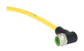
Murrelektronik connection cable, 7/8in - 16 UN2 90-degree male with male threads to Pigtail with European Color Code, 4-pole, 600 VAC/VDC, 9A, 16 AWG, TPE jacket, yellow, unshielded, 16.4ft/5m cable length, IP68, power.
