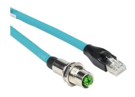
Murrelektronik Cat6a Ethernet bulkhead connector, M12 axial female X-coded 8-pin to RJ45 axial male 8-pin, shielded, 26 AWG, 3.2ft/1m cable length, HDPE conductor insulation material, IP67 (M12) IP20 (RJ45).
