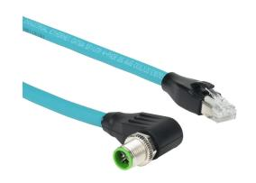
Murrelektronik Cat6a Ethernet connection cable, M12 90-degree male X-coded to RJ45 axial male, 8-pole, 60 VDC, 1.5A, 26 AWG, TPE jacket, teal, overall aluminum foil and tinned copper braid, 32.8ft/10m cable length, IP67 (M12) IP20 (RJ45), data.
