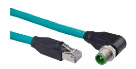
Murrelektronik Cat6a Ethernet straight-through patch cable, overall shielded with foil/unshielded twisted pair, M12 right-angle male X-coded to RJ45 male, 16.4ft/5m cable length, teal. For use with 1/10 Gbps networks.
