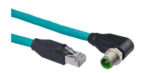
Murrelektronik Cat6a Ethernet straight-through patch cable, overall shielded with foil/unshielded twisted pair, M12 right-angle male X-coded to RJ45 male, 9.8ft/3m cable length, teal. For use with 1/10 Gbps networks.
