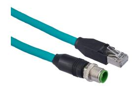
Murrelektronik Cat6a Ethernet straight-through patch cable, overall shielded with foil/unshielded twisted pair, M12 axial male X-coded to RJ45 male, 16.4ft/5m cable length, teal. For use with 1/10 Gbps networks.
