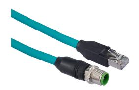
Murrelektronik Cat6a Ethernet straight-through patch cable, overall shielded with foil/unshielded twisted pair, M12 axial male X-coded to RJ45 male, 9.8ft/3m cable length, teal. For use with 1/10 Gbps networks.
