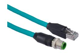
Murrelektronik Cat6a Ethernet straight-through patch cable, overall shielded with foil/unshielded twisted pair, M12 axial male X-coded to RJ45 male, 3.2ft/1m cable length, teal. For use with 1/10 Gbps networks.
