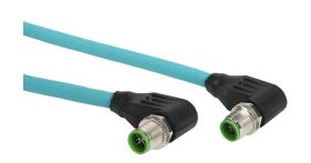
Murrelektronik Cat6a Ethernet connection cable, M12 90-degree male X-coded to M12 90-degree male X-coded, 8-pole, 50 VAC/60 VDC, 0.5A, 26 AWG, TPE jacket, teal, overall aluminum foil and tinned copper braid, 32.8ft/10m cable length, IP67, data.
