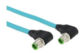
Murrelektronik Cat6a Ethernet connection cable, M12 90-degree male X-coded to M12 90-degree male X-coded, 8-pole, 50 VAC/60 VDC, 0.5A, 26 AWG, TPE jacket, teal, overall aluminum foil and tinned copper braid, 9.8ft/3m cable length, IP67, data.
