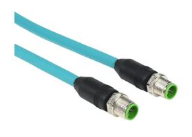
Murrelektronik Cat6a Ethernet connection cable, M12 axial male X-coded to M12 axial male X-coded, 8-pole, 60 VDC, 1.5A, 26 AWG, TPE jacket, teal, overall aluminum foil and tinned copper braid, 32.8ft/10m cable length, IP67, data.
