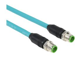
Murrelektronik Cat6a Ethernet connection cable, M12 axial male X-coded to M12 axial male X-coded, 8-pole, 60 VDC, 1.5A, 26 AWG, TPE jacket, teal, overall aluminum foil and tinned copper braid, 16.4ft/5m cable length, IP67, data.
