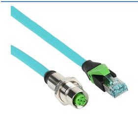
Murrelektronik Cat5e Ethernet straight-through patch cable, STP (overall foil shield), M12 axial female D-coded 4-pin to RJ45 axial male 4-pin, 3.2ft/1m cable length, teal. For use with 10/100 Mbps networks.
