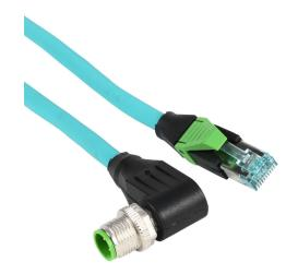
Murrelektronik Cat5e Ethernet straight-through patch cable, STP (overall foil shield), M12 right-angle male D-coded 4-pin to RJ45 axial male 4-pin, 32.8ft/10m cable length, teal. For use with 10/100 Mbps networks.
