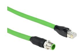
Murrelektronik Cat5e Ethernet connection cable, M12 axial male D-coded to RJ45 axial male, 4-pole, 60 VDC, 1.5A, 22 AWG, TPE jacket, green, overall aluminum foil and tinned copper braid, 49.2ft/15m cable length, IP67 (M12) IP20 (RJ45), data.
