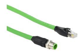
Murrelektronik Cat5e Ethernet connection cable, M12 axial male D-coded to RJ45 axial male, 4-pole, 60 VDC, 1.5A, 22 AWG, TPE jacket, green, overall aluminum foil and tinned copper braid, 16.4ft/5m cable length, IP67 (M12) IP20 (RJ45), data.
