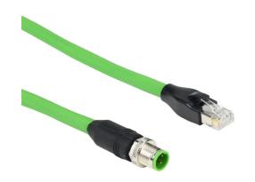
Murrelektronik Cat5e Ethernet connection cable, M12 axial male D-coded to RJ45 axial male, 4-pole, 60 VDC, 1.5A, 22 AWG, TPE jacket, green, overall aluminum foil and tinned copper braid, 9.8ft/3m cable length, IP67 (M12) IP20 (RJ45), data.
