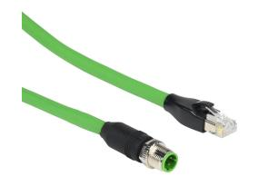
Murrelektronik Cat5e Ethernet connection cable, M12 axial male D-coded to RJ45 axial male, 4-pole, 60 VDC, 1.5A, 22 AWG, TPE jacket, green, overall aluminum foil and tinned copper braid, 3.2ft/1m cable length, IP67 (M12) IP20 (RJ45), data.
