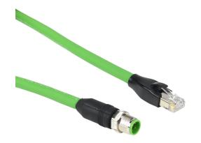
Murrelektronik Cat5e Ethernet connection cable, M12 axial male D-coded to RJ45 axial male, 4-pole, 60 VDC, 1.5A, 22 AWG, TPE jacket, green, overall aluminum foil and tinned copper braid, 1.9ft/0.6m cable length, IP67 (M12) IP20 (RJ45), data.
