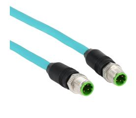
Murrelektronik Cat5e Ethernet straight-through patch cable, STP (overall foil shield), M12 axial male D-coded 4-pin to M12 axial male D-coded 4-pin, 24.6ft/7.5m cable length, teal. For use with 10/100 Mbps networks.
