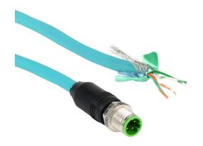
Murrelektronik Cat5e Ethernet connection cable, STP (overall foil shield), M12 axial male D-coded 4-pin to pigtail, 32.8ft/10m cable length, teal. For use with 10/100 Mbps networks.
