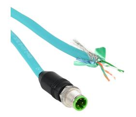
Murrelektronik Cat5e Ethernet connection cable, STP (overall foil shield), M12 axial male D-coded 4-pin to pigtail, 16.4ft/5m cable length, teal. For use with 10/100 Mbps networks.
