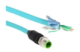
Murrelektronik Cat5e Ethernet connection cable, STP (overall foil shield), M12 axial male D-coded 4-pin to pigtail, 1.9ft/0.6m cable length, teal. For use with 10/100 Mbps networks.
