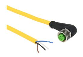
Murrelektronik connection cable, M12 90-degree female A-coded to pigtail, 4-pole, 250 VAC/VDC, 4A, 22 AWG, TPE jacket, yellow, unshielded, 32.8ft/10m cable length, IP65 IP66K IP67, sensor & signal.
