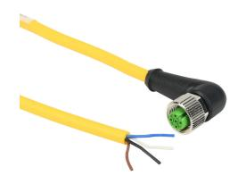
Murrelektronik connection cable, M12 90-degree female A-coded to pigtail, 4-pole, 250 VAC/VDC, 4A, 22 AWG, TPE jacket, yellow, unshielded, 9.8ft/3m cable length, IP65 IP66K IP67, sensor & signal.
