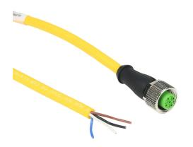
Murrelektronik connection cable, M12 axial female A-coded to pigtail, 4-pole, 250 VAC/VDC, 4A, 22 AWG, TPE jacket, yellow, unshielded, 16.4ft/5m cable length, IP65 IP66K IP67, sensor & signal.
