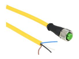
Murrelektronik connection cable, M12 axial female A-coded to pigtail, 4-pole, 250 VAC/VDC, 4A, 22 AWG, TPE jacket, yellow, unshielded, 9.8ft/3m cable length, IP65 IP66K IP67, sensor & signal.
