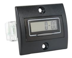
Trumeter electrical hour meter, 9mm 8-digit LCD, discrete input, remote, manual or disabled reset, rectangular flush mount with clip, screw terminals.
