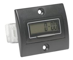
Trumeter electrical hour meter, 9mm 8-digit LCD, 5-110 VDC or 10-240 VAC input, remote, manual or disabled reset, rectangular flush mount with clip, screw terminals.
