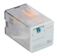
AutomationDirect octal control relay, socket mount, encapsulated push-to-test, 12 VDC coil voltage, 3PDT, (3) N.O., (3) N.C., 10A contact rating, 11-pin, LED indicator(s). Requires 750-3C-SKT mounting socket.
