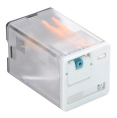
AutomationDirect octal control relay, socket mount, encapsulated push-to-test, 24 VDC coil voltage, DPDT, (2) N.O., (2) N.C., 10A contact rating, 8-pin, LED indicator(s). Requires 750-2C-SKT mounting socket.
