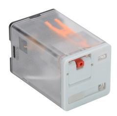
AutomationDirect octal control relay, socket mount, encapsulated push-to-test, 24 VAC coil voltage, DPDT, (2) N.O., (2) N.C., 10A contact rating, 8-pin, LED indicator(s). Requires 750-2C-SKT mounting socket.
