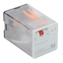
AutomationDirect octal control relay, socket mount, encapsulated push-to-test, 240 VAC coil voltage, DPDT, (2) N.O., (2) N.C., 10A contact rating, 8-pin, LED indicator(s). Requires 750-2C-SKT mounting socket.
