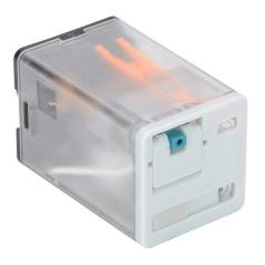
AutomationDirect octal control relay, socket mount, encapsulated push-to-test, 12 VDC coil voltage, DPDT, (2) N.O., (2) N.C., 10A contact rating, 8-pin, LED indicator(s). Requires 750-2C-SKT mounting socket.
