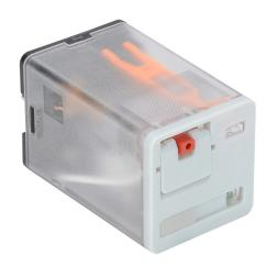
AutomationDirect octal control relay, socket mount, encapsulated push-to-test, 12 VAC coil voltage, DPDT, (2) N.O., (2) N.C., 10A contact rating, 8-pin, LED indicator(s). Requires 750-2C-SKT mounting socket.
