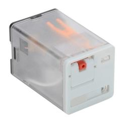
AutomationDirect octal control relay, socket mount, encapsulated push-to-test, 120 VAC coil voltage, DPDT, (2) N.O., (2) N.C., 10A contact rating, 8-pin, LED indicator(s). Requires 750-2C-SKT mounting socket.
