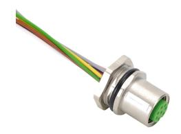
Murrelektronik bulkhead connector, M12 8-pin female to pigtail, 24 AWG, 3.2ft/1m cable length, nylon 12 conductor insulation material, IP67.
