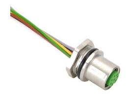
Murrelektronik bulkhead connector, M12 nut 8-pin female to pigtail, 24 AWG, 3.2ft/1m cable length, polypropylene conductor insulation material. Mounting nut(s) included.
