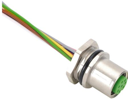
Murrelektronik bulkhead connector, M12 8-pin female to pigtail, 24 AWG, 3.2ft/1m cable length, nylon 12 conductor insulation material, IP67.
